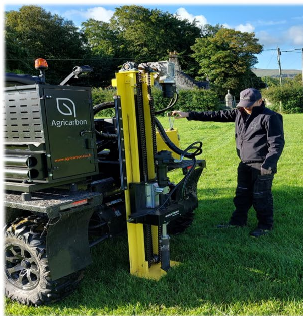
Soil Sampling to one metre deep
