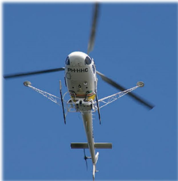
Aerial LiDAR Survey at 40 scans per metre
